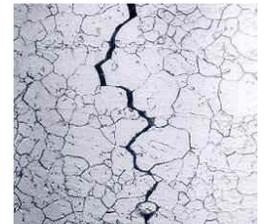
Microscopic stress corrosion crack
