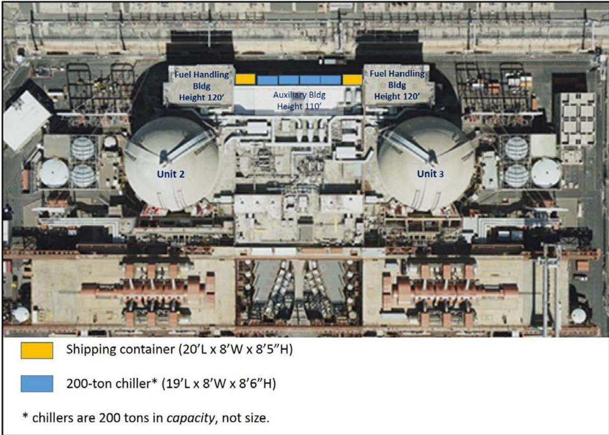
**Above:** Configuration of the shipping containers and chillers between the Units 2 and 3 fuel handling buildings (Note: shipping container and chiller representations not to scale; the area that will be occupied is less than half the space shown in this figure)
