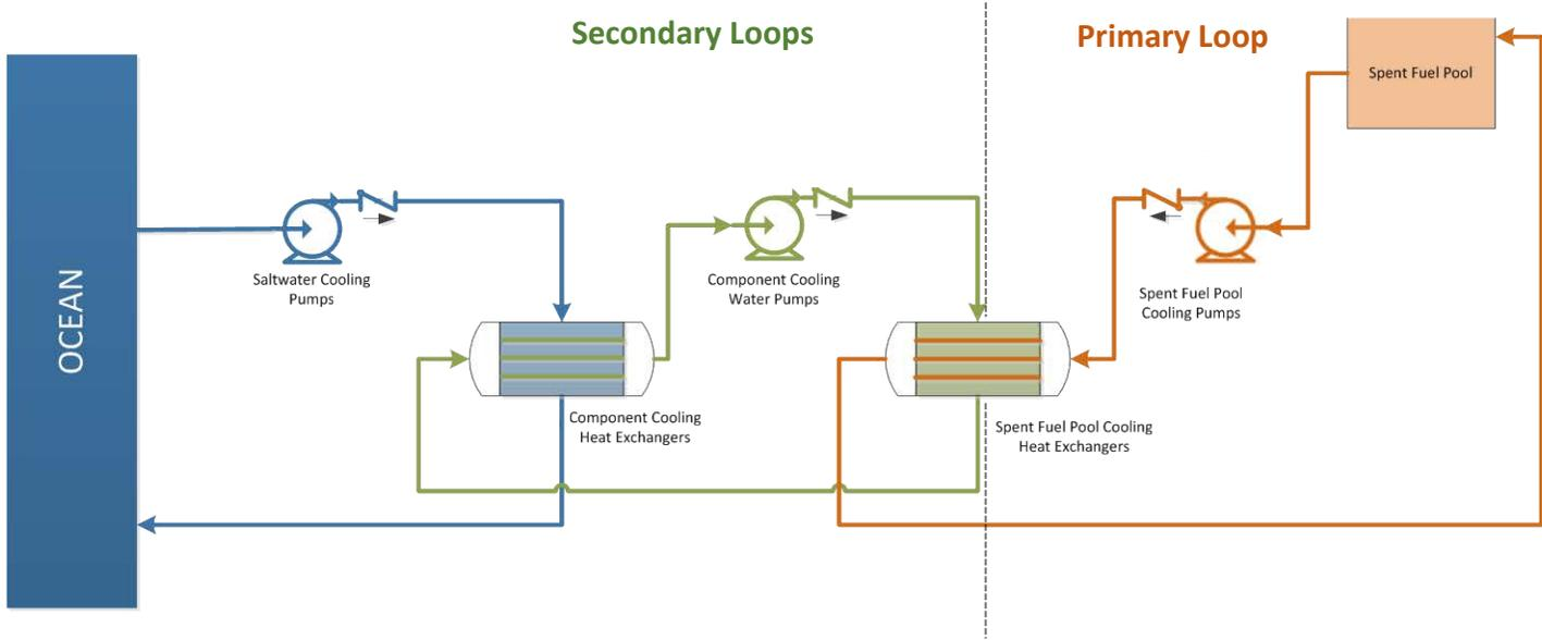
**(B) Schematic of Proposed Spent Fuel Pool Island Cooling System**
