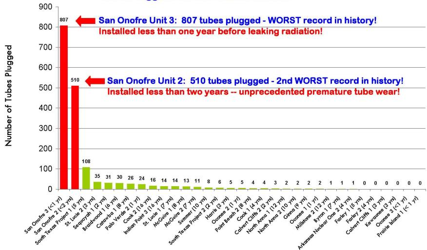
Nuclear Reactors (years of replacement steam generator operation before tubes plugged)
