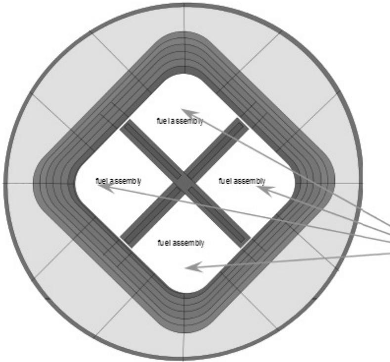
**Fig. 1. Cross-section of the GA-4 cask, including the propylene neutron absorber.**
