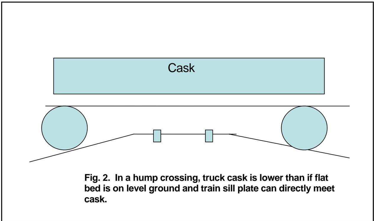
My conclusion from the Ammerman study is that the forces on the cask bolts would exceed yield and the cask lid would open and remain open. Further, the fuel rods would break ("shatter" is a more appropriate description) and release gases and semi-volatile radionuclides, such as Cs. Far from supporting the conclusion of NUREG-2125 that no material would be released in a truck/locomotive accident, this reference contradicts it.
