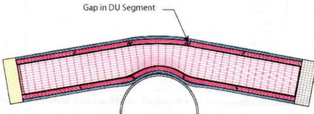
**Figure 34. GA-4 cask after 96 kph [60 mph] back-breaker impact.**
