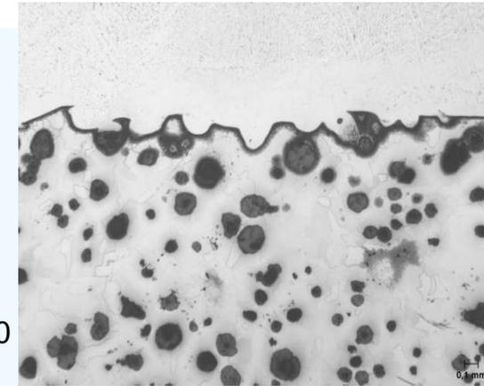
Microstructure of welded zone
