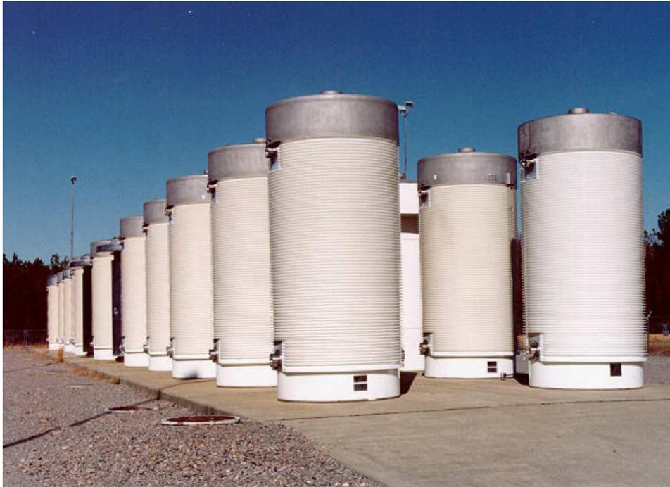
Open air storage by INEEL of CASTOR® V/21
