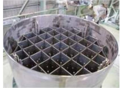
37 fuel assembly thin-wall canister
