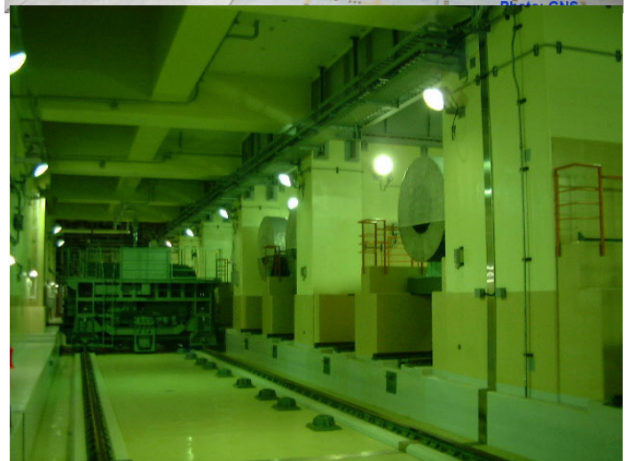
Transport and storage casks in the interim storage facility of Gorleben
