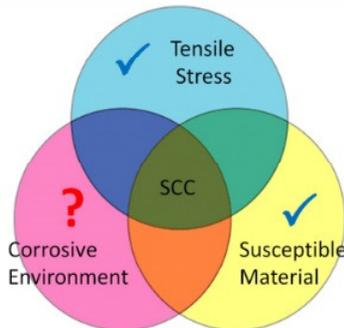
**2/3 of the requirements for SCC are present in welded stainless steel canisters**
